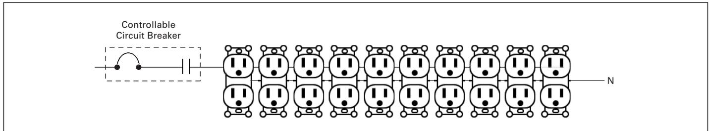
Figure 4. Receptacle Control Using Controllable Circuit Breaker
