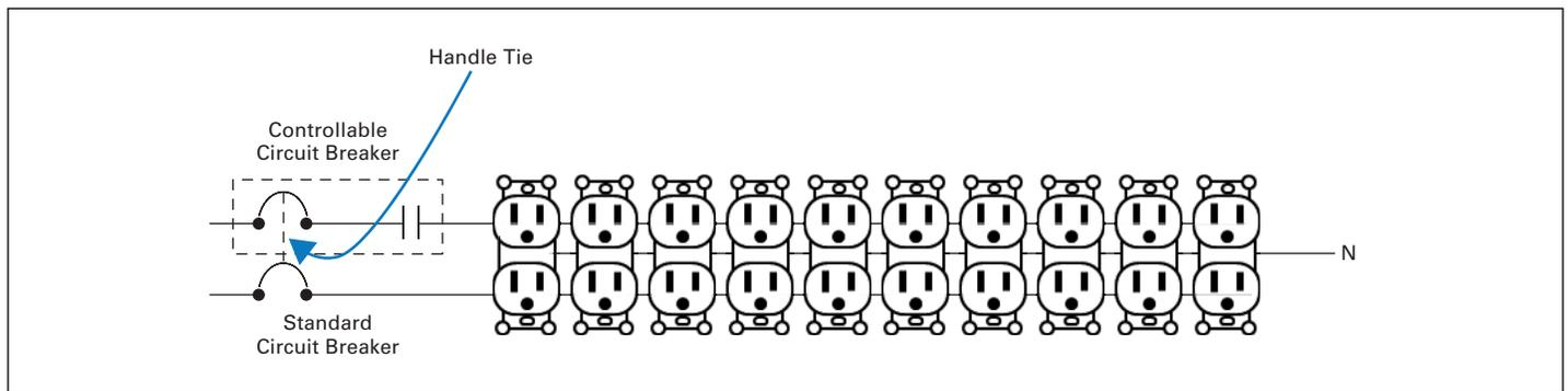
Figure 5. Split Receptacle Control Using Controllable Circuit Breakers
