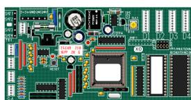
Provides control for 4 zones in a multi-zone system. Each zone has a thermostat with 10k thermistor, adjustable setpoint, and override switch. (Does not support thermostat LED or LAN connection.) Each zone also has an actuator with feedback status and a sensor indicating mixed supply air temperature. The application-specific intelligence built into the Multi-zone board is designed to operate with a UUC-8S that controls the Multi-zone air handler.
