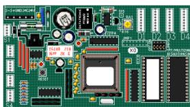
Provides control for 4 VVT zones. Each zone has a thermostat with 10k thermistor, adjustable setpoint, and override button. (Does not support thermostat LED or LAN connection.) Each zone has an actuator with feedback status. The application-specific intelligence built into the VVT board is designed to operate with a UUC-8S that controls the roof top unit and bypass damper. All VVT zones and the UUC-8S are scheduled and function together as a single system.
